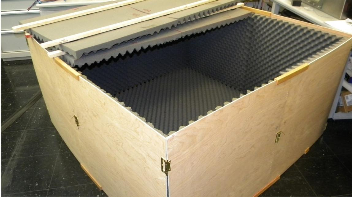
Figures 5.3. Inside of View of the Acoustic Chamber from the Top
