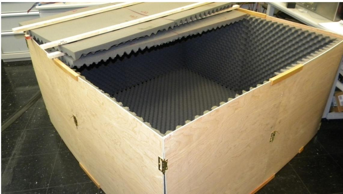
Figures 5.3. Inside of View of the Acoustic Chamber from the Top
