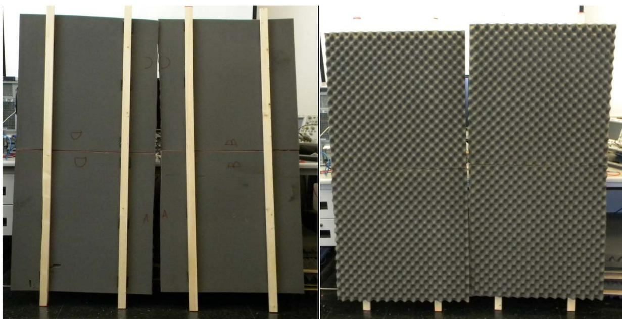
Figures 5.6. Acoustic Chamber Ceiling Tiles Front and Back
