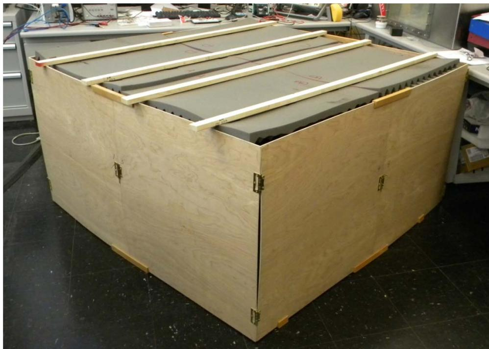
Figures 5.1. Outside of View of the Acoustic Chamber from the Top
